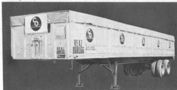
Special low-sided open-top trailers with removable sides , ideal for marble, steel, heavy parts . . . offer ease of loading and unloading with lift equipment. Tarpaulin protection.
