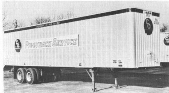
Special insulated all-weather trailers are Chessie's answer for dry-van products that need protection against critical temperature changes while in transit.
