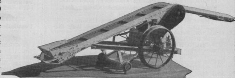
The Mount Vernon Pit Car Loader Is of Light, Sturdy Construction, Easily Moved Off and On Tracks and About Rooms. Weight—Only 1200 to 1600 Lbs.—Has Been Carefully Balanced on Roller Bearing Wheels so That One Man Can Move it with Ease on the Rails, or on a Hard, Smooth Bottom
