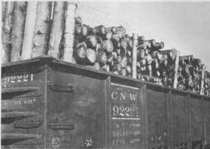
Fig. 4 Properly loaded and wired car of peeled pulpwood.
